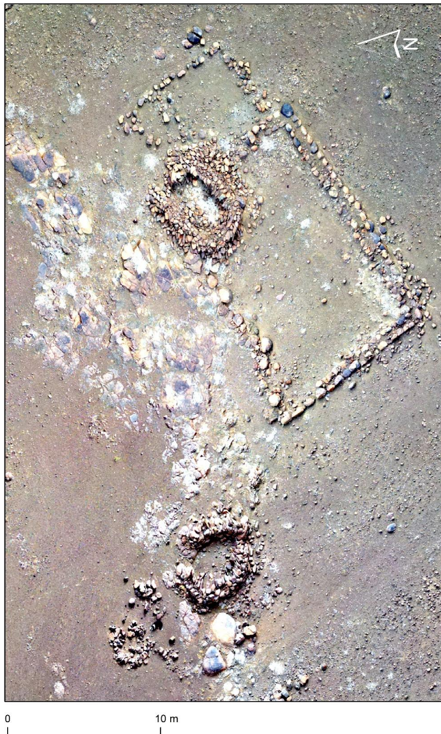
Figure 10: Orthophoto image of the main drystone structures at QRS 10/44. Note the construction method in the outer rectangular wall employing a single outer and inner course with through-band stones and filled with coarse rubble, a common early colonial drystone building technique.
